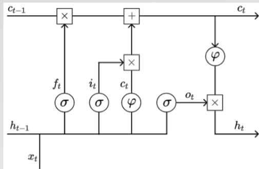
**Long Short-Term Memory (LSTM):** LSTM is a gated RNN (Recurrent Neural Network). There are 4 gates and a cell state ( $\mathbf{c}_t$ ): hidden gate ( $\mathbf{h}_t$ ), input gate ( $\mathbf{i}_t$ ), forget gate ( $\mathbf{f}_t$ ), output gate ( $\mathbf{o}_t$ ).
