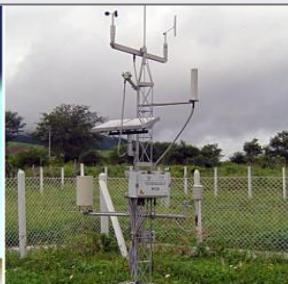
Picture 3. Automatic Data Collection Station (Brazilian Solar Energy Atlas, 2017).
